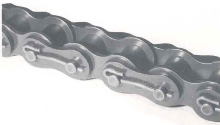
Most bushings, rollers, rivets and pins for the Link-Belt® FR® chain are manufactured using a cold forming process. Cold forming imparts to the metal a more refined and homogeneous grain structure. Combined with specific heat-treating processes, this results in improved mechanical and fatigue properties, as well as higher wear resistance.
